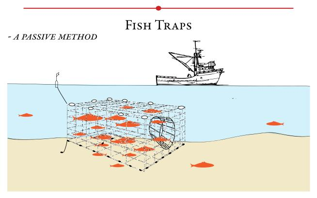
Fish traps are large net or link traps suspended in the water or on the bottom, marked by buoys, weighted, and anchored. Fish are able to swim in, small size fish can escape and non-targeted fish can be released alive when the fishermen return to harvest the targeted fish.
