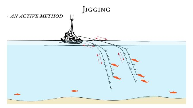
Jigging is the setting of a line, with baited hooks or lures, that is continually jerked. The motion, achieved by hand or with a jigging machine, induces fish, such as cod and squid, to take the hook.
