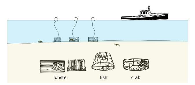
Pots or traps are often designed specifically for one type of fish or shellfish. Traps and pots are generally baited and equipped with one or more funnel openings, and they are weighted to rest on the bottom. Pots or traps can be fished singularly or in small groups, and each has a buoy at the surface to mark location.
