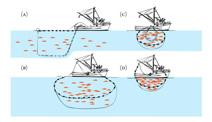
Purse seines are walls of netting used to encircle entire schools of fish such as sardines, mackerel, squid, and some tuna, at or near the surface. A drawstring cable is threaded through the bottom of the net. When the cable has pulled the netting tight, enclosing the fish in a pouch, the catch is hauled onboard with a dip net in a process called brailing.
