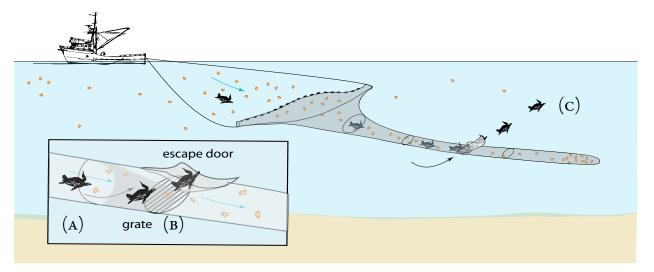
Turtle extruder devices are net modifications consisting of grates that are sewn into nets adjacent to open flaps that function as escape hatches.
