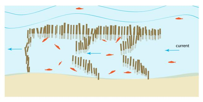
Weirs are constructions designed from branches or stones that impede free movement of fish such as mackerel and herring by obstructing running waters, and then guiding fish into cordoned areas as they migrate.
