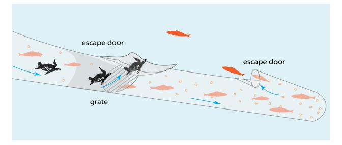
A bycatch reduction device is an opening in a shrimp trawl net that allows finfish or other sea animals to escape, while the target species of shrimp is directed towards the bag end of the net. BRDs are required in shrimp trawl nets in federal waters of the Gulf of Mexico and South Atlantic regions.
