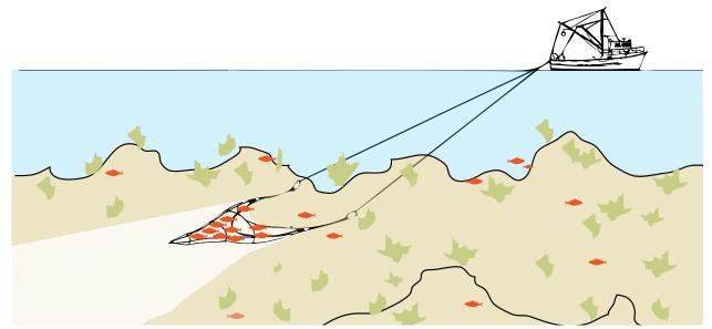
Rocky Bottom Trawling or Dragging is the method of fishing responsible for the greatest environmental damage. This trawling drags a net weighted down with extremely heavy cables and rollers over the ocean floor, scraping everything in its path, including all sea creatures and plant life-forms, as well as the habitat necessary for their survival. TURTLE EXTRUDER DEVICES - T.E.D.S - FOR SHRIMP TRAWLERS - ACTIVE METHOD
