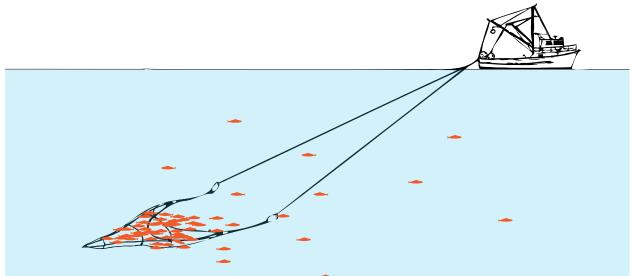
Trawling or Dragging is the method of fishing responsible for the greatest percentage of fishery landings. Trawling is simply described as towing a net through water. Mid-water trawlers tow a funnel-shaped net through the water column between the surface and the bottom, targeting mid-level pelagic fish, such as true cod and pollock, resulting in less impact on fishery habitat and less bycatch.
