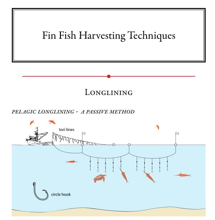
Longlining uses baited hooks, on offshoots of a single main line, to catch fish at any depth. The line can be anchored in areas too rough for trawling, or set adrift, suspended by floats.
